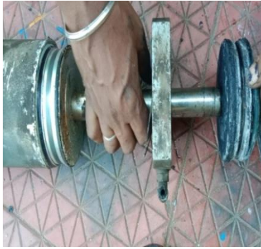
Piston Disc (Air side) found good and intact
