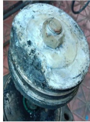
Piston Disc (Water side) found decayed
